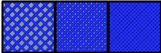
Fig. 1 Variety of infill rectilinear patterns available to print in slic3r. Left to Right: 40%, 70%, 100%.
