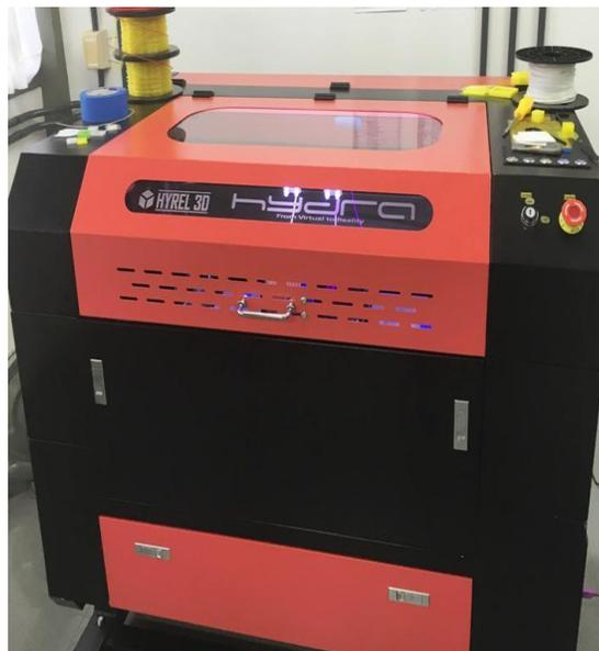
**Figure 5: The LACESM/CT-UFSM's 3D Printer "Hyrel Hydra" used**
