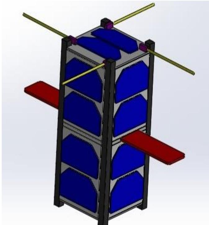
**Figure. 4: NCBR2 CAD Model in Solid-works environment**
