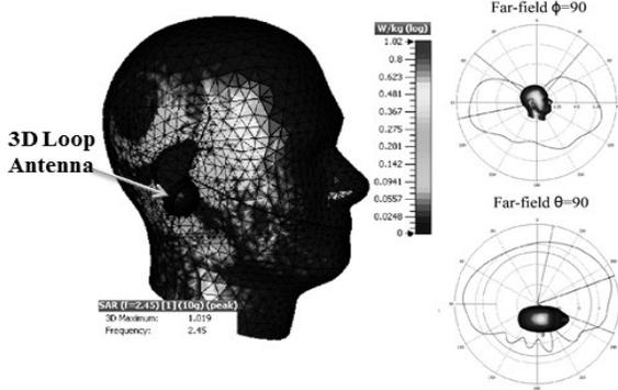
Fig. 6 Simulated SAR values and the radiation pattern for an ear-mounted 3-D loop antenna configuration
