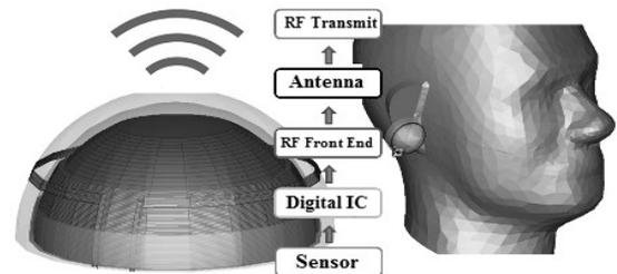
Fig. 1 3-D packaging for health monitoring and IoT applications
