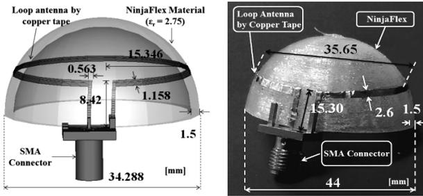
Fig. 2 a) Optimized simulation model of the loop antenna in CST Microwave Studio, b) Fabricated 3-D loop prototype antenna with dimensions after tuning
