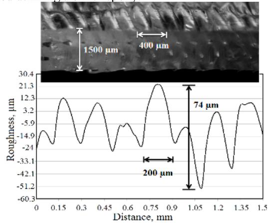
Fig. 3 Profilometer measurement compared with microscopic cross section photo of the NinjaFlex ring
