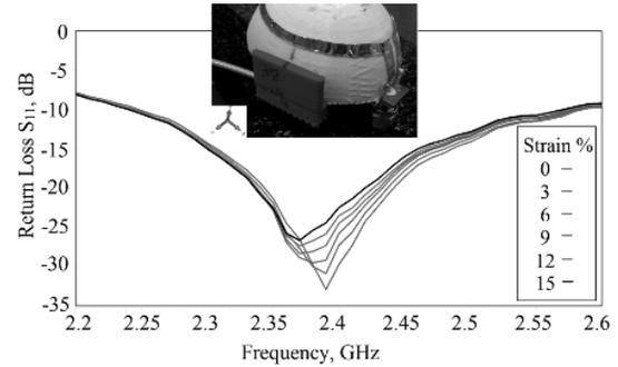
Fig. 7 Measured return loss of the loop antenna under different strain percentages
