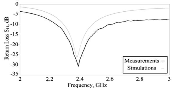
Fig. 5 Return loss  $S_{11}$  of the loop antenna prototype
